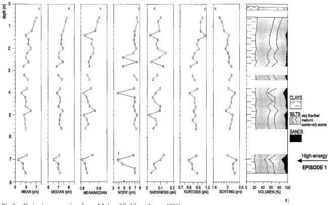
Fig. 3. Grain size properties of core LL (modified from LARIO 1996).
