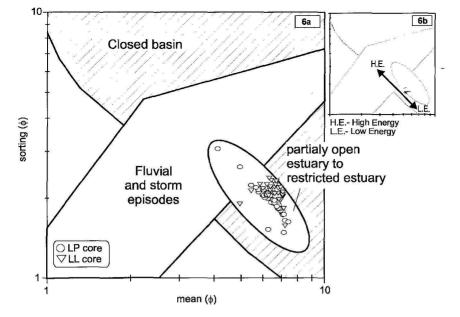
Fig.6 a) Diagram of mean grain size versus sorting of sediments from cores LL and LP (modified from LARIO 1996). The sedimentary environments are modified from the classification of TANNER (1991). b) This should be also interpreted in terms of changes in the hydrodynamic conditions and energy of the depositional environment.
