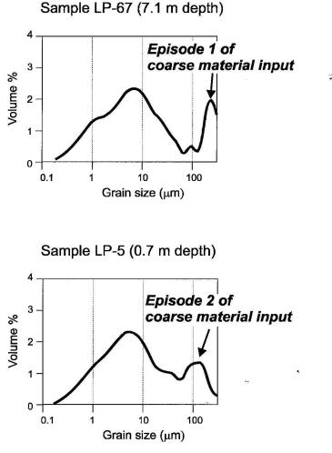
Fig. 7. Diagram of particle size analyses distribution of episodes identified in fig. 2. The bimodal distributions reflect the input of coarse sediment (arrows) associated with the high energy of these events.
